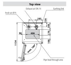
Diagram shows left-hinged door. Dimensions are identical for a right-hinged fitting.
