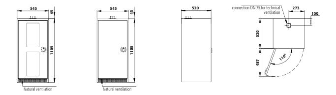
Diagram shows left-hinged door. Dimensions are identical for a right-hinged fitting.
